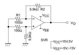
$$SVR(+)=20log \left| \frac{\Delta V_{CC} \times 100}{\Delta V_{O}} \right|$$
